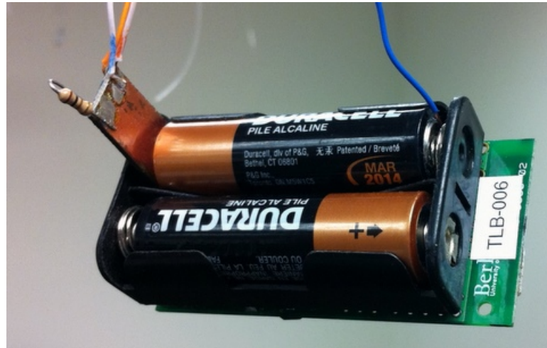
Figure 2.7: The energy monitoring circuitry. A small PCB board, on which a 1-Ohm resistor is soldered on, is used to insert the resistor into the note circuitry.
